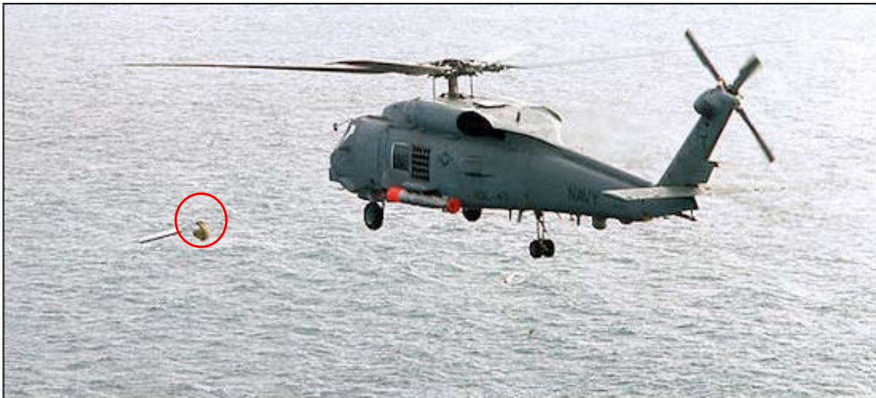
Figure 3.0-2: Sonobuoy Launch Depicting the Relative Size of a Small Decelerator/Parachute
