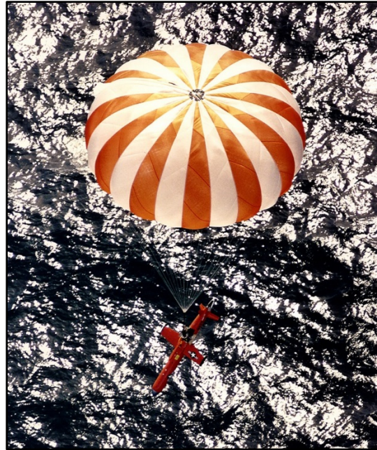
Figure 3.0-3: Aerial Target (Drone) with Parachute Deployed
