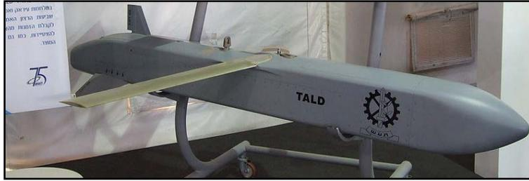
**Figure A-3: Tactical Air-Launched Decoy (Aerial Target)**
