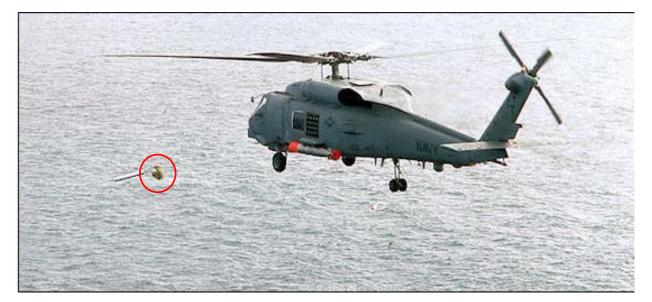
Figure 3.0-1: Sonobuoy Launch Depicting the Relative Size of a Small Decelerator/Parachute
